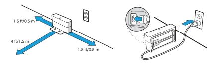
MARNING: To prevent the risk of your robot falling down stairs, ensure that the charging station is placed at least 4 feet (1.2 metres) away from stairs.
